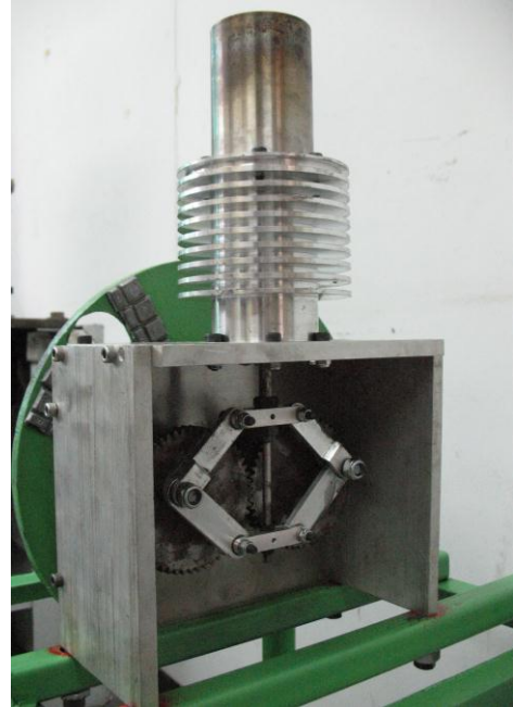
Fig. 3 The rhombic- drive Stirling engine prototype
