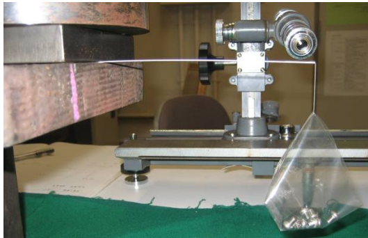
Fig. 10 View of bending test
