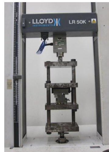
Fig. 5 Wipe bending die set on universal tensile testing machine
