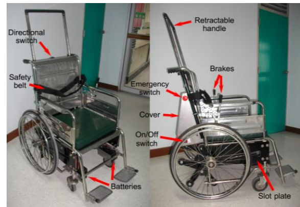
Fig.10 Wheelchair equipped with the stair-climbing system
