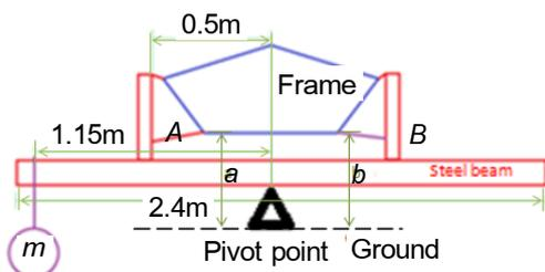
Figure 18 Torsional test (rear view)
