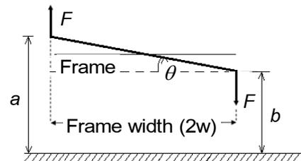
Figure 20 The twist angle
