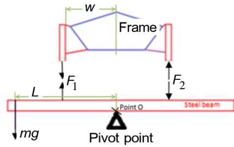
Figure 19 Forces acting on the frame
