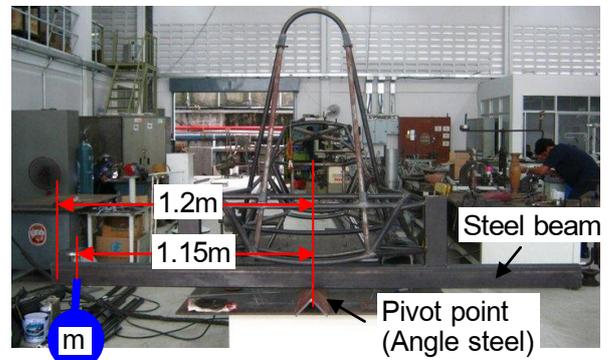
Figure 21 Beam construction on the rear
