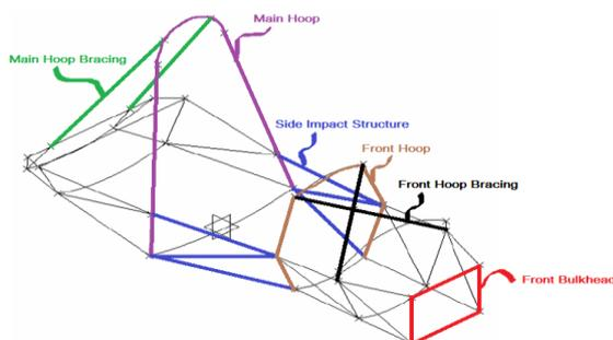
Figure 3 Definitions of frame's parts
