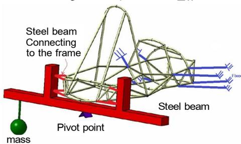
Figure 17 Torsional test
