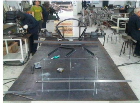
Figure 8 Guide drawing on the flat steel table
