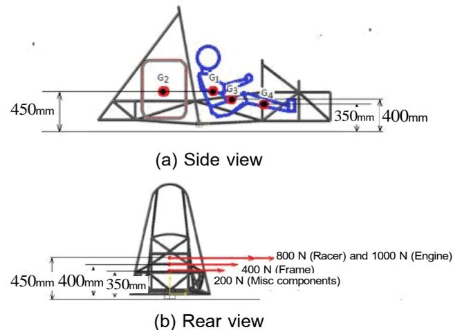
Figure 1 Center of gravity and forces on car
