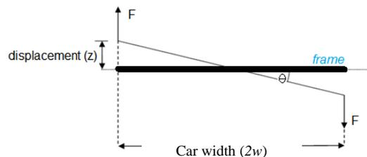
Figure 2 Angle of twist
