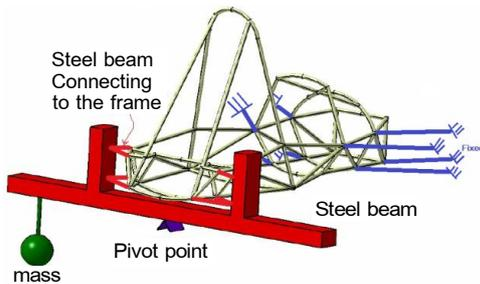
Figure 17 Torsional test
