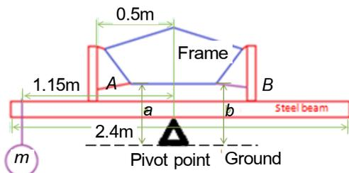
Figure 18 Torsional test (rear view)
