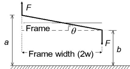
Figure 20 The twist angle
