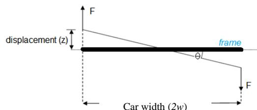
Figure 2 Angle of twist
