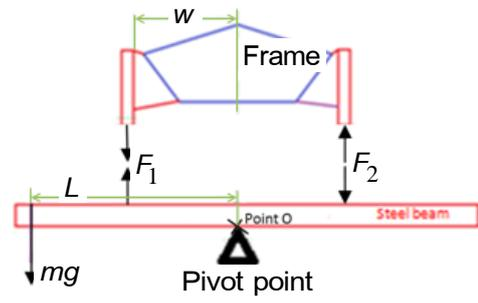
Figure 19 Forces acting on the frame
