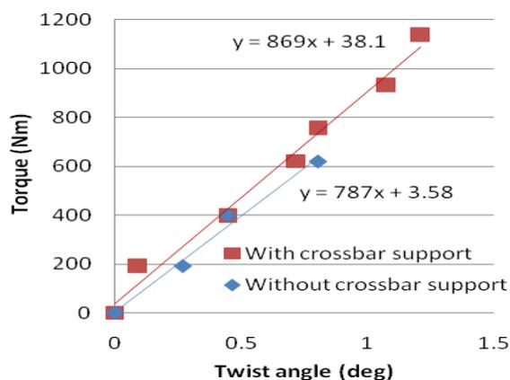
Figure 23 Torsional stiffness from test
