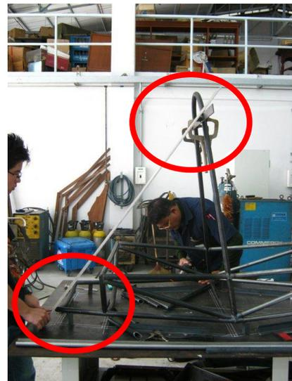
Figure 15 The angle of the main hoop bracing
