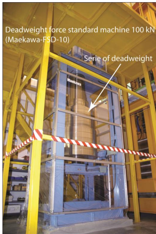
Fig. 1 NIMT's Deadweight force machine 100 kN
