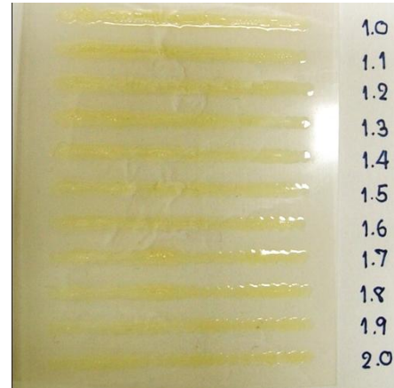
Fig.7 The printed lines of the first chemical group with droplet pitch 1.0 - 2.0 mm.
