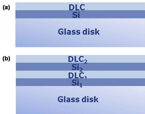
Fig. 9 The disk configurations which are proposed to improve the sensitivity: (a) 2-layer coated disk; (b) 4-layer coated disk
