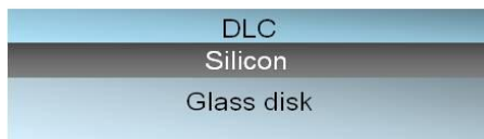
Fig. 2 The schematic illustration of the glass disk coated with silicon and DLC layers.
