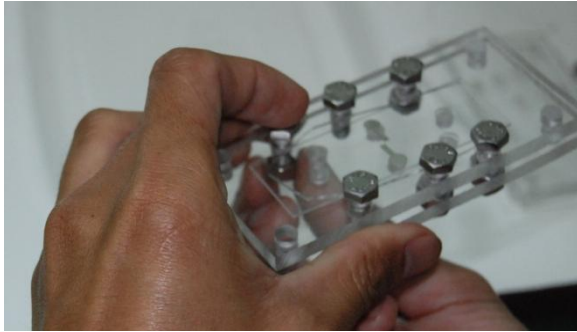
Fig. 5 The LOC fabricated at Kasetsart University, Chalermphrakiat Sakon Nakhon Province Campus
