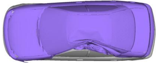
Fig. 17 Top view of Chrysler Neon overlapping pre (gray) and post (purple) impact
