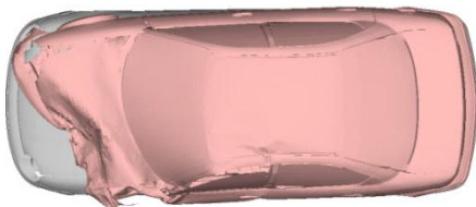
Fig. 9 Top view of Chrysler Neon overlapping pre (gray) and post (pink) impact
