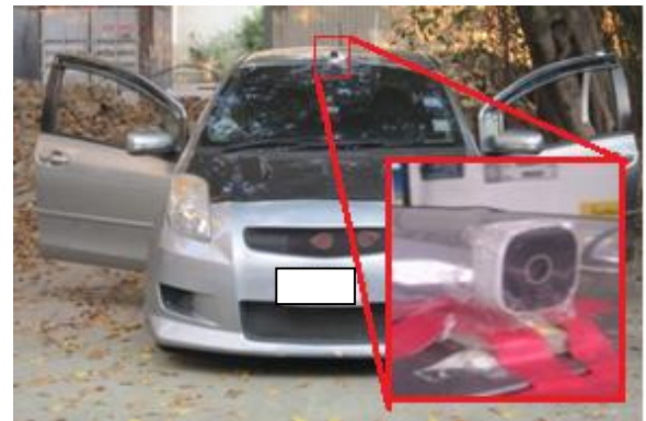
Fig. 6 webcam for detecting headway distance
